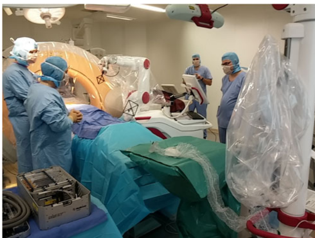
Fig. 1 A view of the operating theater after draping under sterile conditions. The O-arm® flat-panel CT device is placed to the left of the surgeon and the ROSA™ SPINE robot is placed facing the surgeon and slightly to his left. The robot's specific fiducial marker and stereoscopic camera are located slightly to the right of the surgeon
