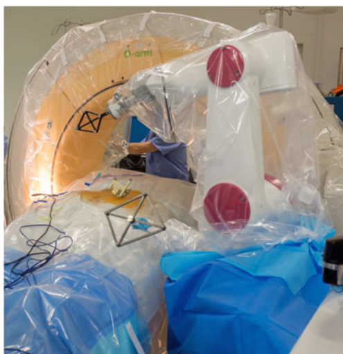
Fig. 2 A close-up view of the robot's fiducial marker. This enables the robot to monitor its own movements in real time. This further improves safety by merging these data with information from the iliac crest fiducial marker
