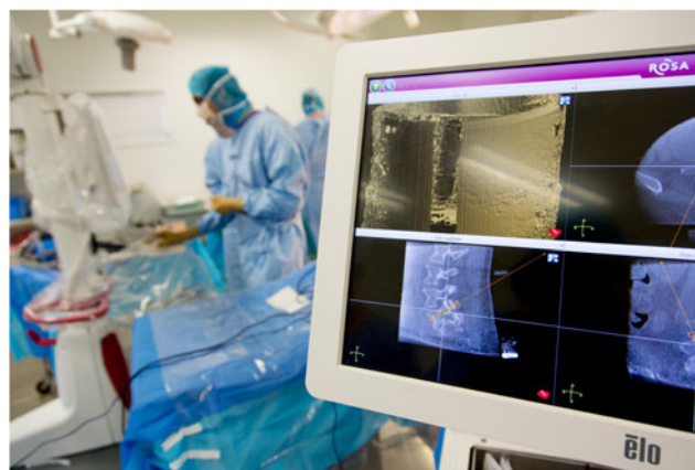
Fig. 4 The surgeon chooses the entry and end points, the trajectories, and the screw diameter using the robot's software. The robot's display screen shows the entire trajectory in three dimensions
