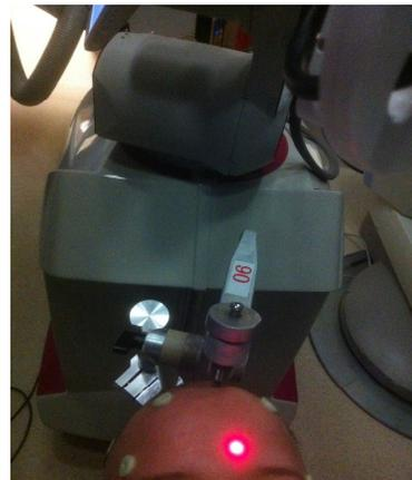
**Figure 3:** Automated laser based surface registration. When positioning needs dictate that the face be inaccessible to the robotic arm, fiducial based registration can alternatively be used.
