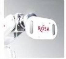
In July 2014, MEDTECH obtained the CE marking for its new product ROSA™ Spine, a robotic- assistive device for minimally invasive surgery of the spine.
